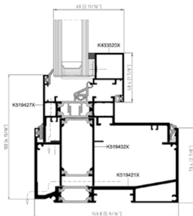
Operable window SG, sill receptor cross-section
