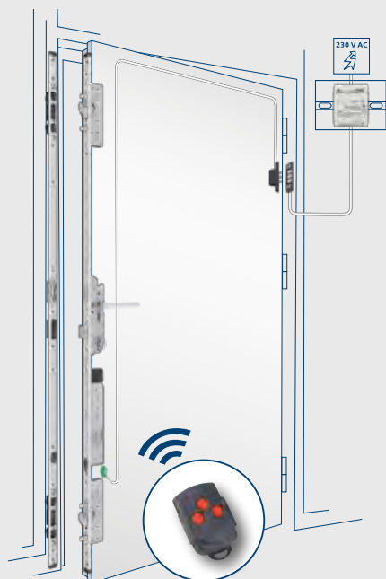
Mains adapter for rail mounting plus radio receiver module
